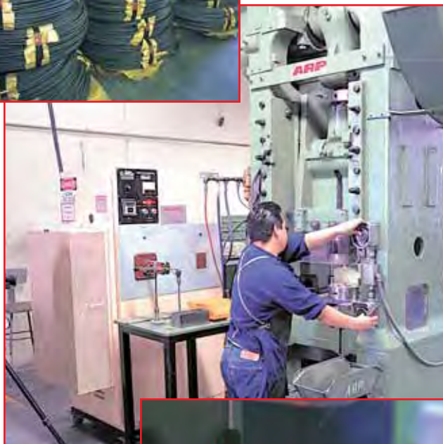
Material comes from the mill in large coils...which subsequently will be fed into cold-headers and formed into bolts.
