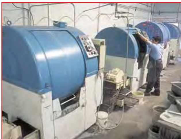
ARP's popular stainless steel engine & accessory fasteners are polished to a brilliant luster using this specialized equipment.
