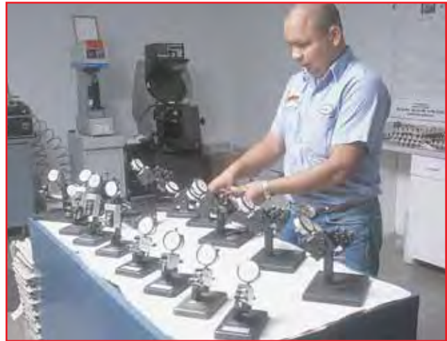
A series of special checking devices are employed to monitor the quality of threads. For every thread size, there is a checking device.
