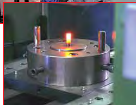
Some bolts begin as induction-heated lengths of bar stock that are forged on huge presses with the desired head shape.
