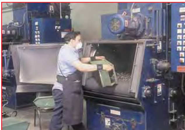
Fasteners are shot-peened after heat-treatment to remove any surface irregularities and improve overall external integrity.
