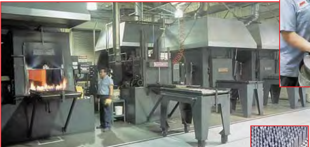
Heat-treating is critically important in obtaining the correct tensile strength. Fasteners are placed in special vertical racks to ensure complete 360° penetration.
